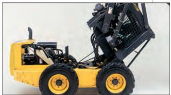
Loader boom-locks that you engage from inside the cab allow you to secure the raised boom before you get out to perform scheduled maintenance. LS Super Boom loader arms pivot on the either 51 or 64 diameter pins. These are induction hardened and have an integral spiral lubrication channel machined into their surface. This traps lubricant and enables routine greasing to be extended to 50 hour intervals.
