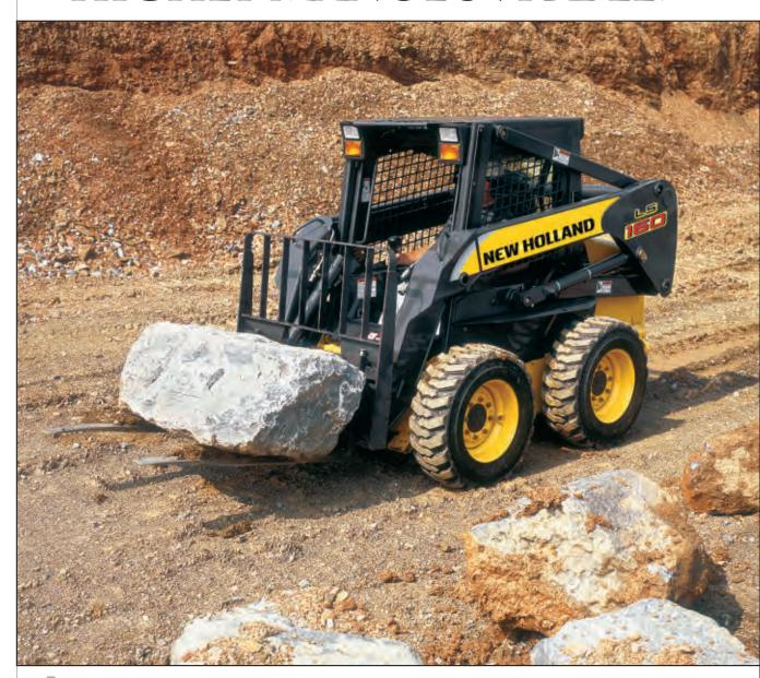
skid-steer loader has to be able to turn within its own length, but it also needs to be stable. Stable enough to give operators the confidence to quickly exploit the machine's full lift capacity. New Holland LS skid-steer loaders have a long wheelbase and an exceptionally low centre of gravity. Compared with a traditional skid-steer, LS Super Boom skid-steers are:
